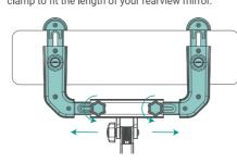
7. Install the rearview mirror car mount onto the rearview mirror, and then press the telescopic clamp arms fixed button to lock the rearview mirror
